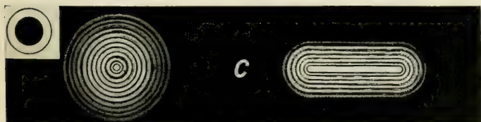
FIG. 60 c shows the image formed by an annular-ring aperture when inner and outer diameters are \cdot 65 N.A. and \cdot 5 N.A. The central spot is small, but the rings, or some of them, are almost as bright as the central spot, and the result on the image of a line is almost as bad as that of a small aperture. The brilliancy of the surrounding rings is dependent on the width of the annular aperture. The smaller the thickness of the annular ring the more brilliant the lines. Therefore, this form of aperture is not usually satisfactory.
